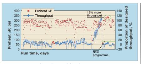
Figure 5 Lower pressure drop and increased throughput
