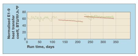
Figure 3 Improved heat transfer on exchanger bundle 4
