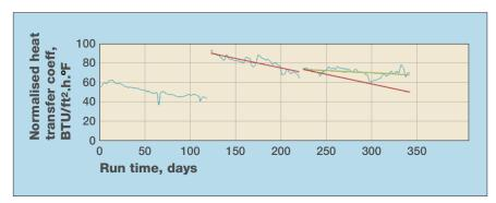
Figure 2 Improved heat transfer on exchanger bundle 2
