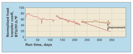
Figure 1 Improved heat transfer on exchanger bundle 1
