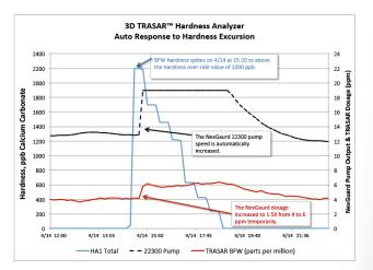
Figure 2 - 3D TRASAR Technology for Boilers System automatically responds to the upset condition.
